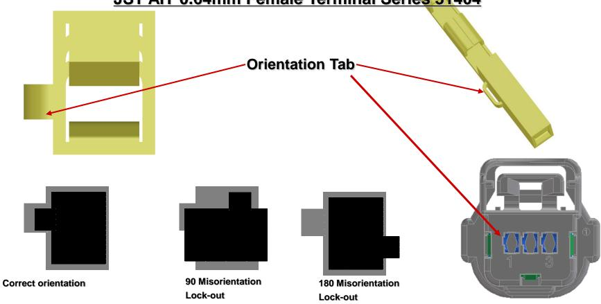
**Terminal Insertion Orientation to Grommet Seal Cover**
