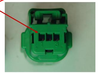
**Terminal Insertion Orientation to Grommet Seal Cover**
