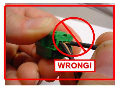
If the wire insulation is pierced or chafed. This may create a leakpath for fluid ingress and/or wire corrosion.
